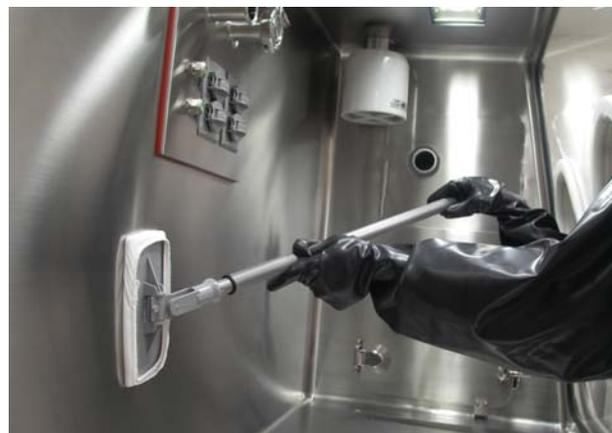
Figure 1. Isolator cleaning tool in use
