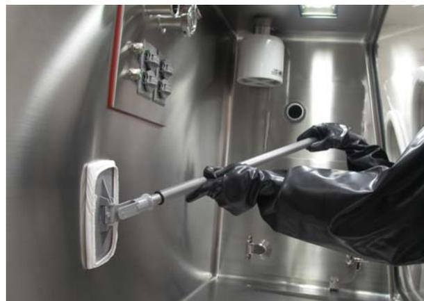
Figure 1. Isolator cleaning tool in use
