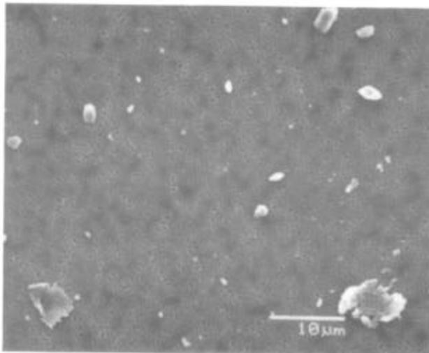
Figure 4: SEM micrograph at 2000x showing particle release from wiper D when subjected to orbital shaking in an IPA/DI-water solution.
