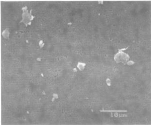
**Figure 3: SEM micrograph at 2000× showing particle release from wiper D when subjected to orbital shaking in a surfactant/DI-water solution.**
