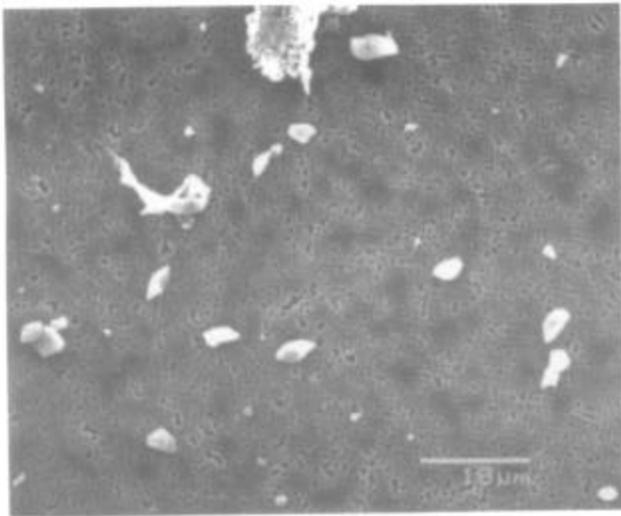
**Figure 2: SEM micrograph at 2000x showing particle release from wiper D when subjected to minimal stress in a surfactant/DI-water solution.**
