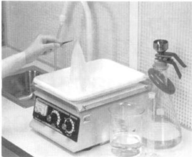
**Figure 1: Applied mechanical energy test setup using an orbital shaker to agitate the wiper.**
