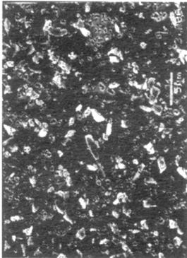
COVER PHOTO: SEM (Scanning Electron Microscopy) utilized as a metrology tool of choice for the counting and analyzing of particles and fibers. This 3000X photomicrograph, taken at Texwipe's Research and Development Laboratory, shows particle distribution on a polycarbonate membrane filter. Photo used courtesy of Texwipe.
