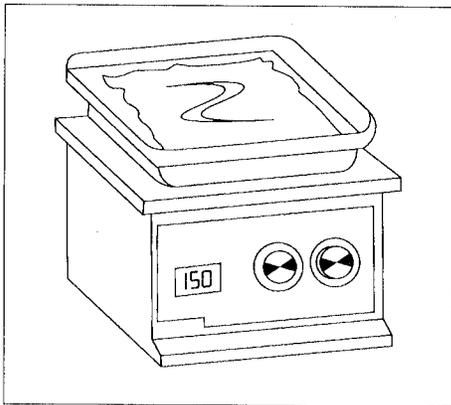
Figure 1. Test setup using an orbital shaker to agitate the wiper.
