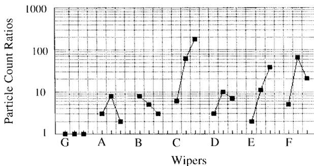
*Figure 7. Semilog plot of the ratio of particle counts for all wipers, as determined by microscopy at various magnifications. For each wiper, the first number (from left) is at 20X, the second is at 200X, and the third is at 3000X.*
