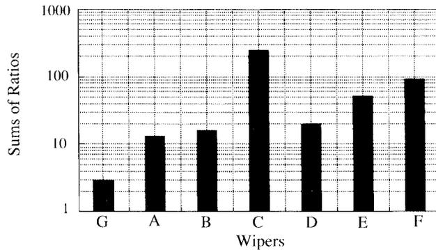
Figure 8. Semilog plot of the total contamination index for all wipers.
