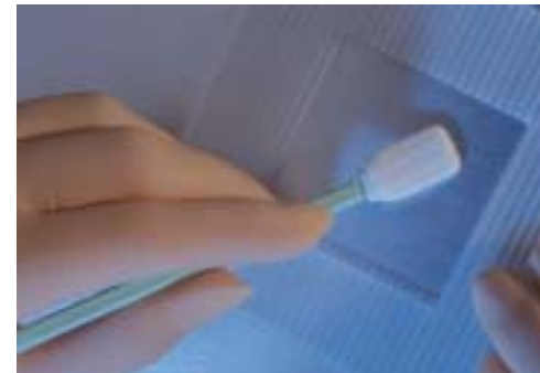
Fig. 2 — Swab with entire head flat against testing surface
