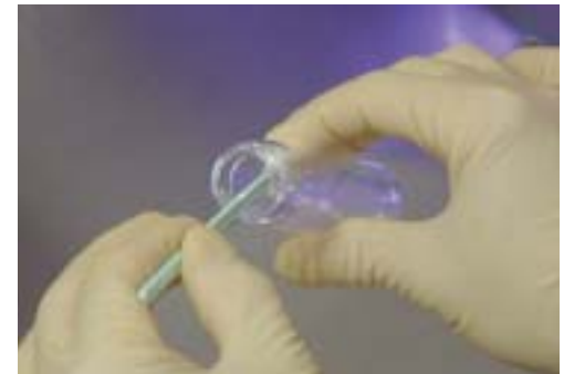
Fig. 3 — Snap swab head at the notch along narrow edge of swab handle
